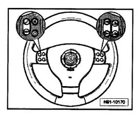
The multi-function steering wheel allows some functions of the Communication system to be operated from the steering wheel.
